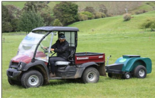
To use, you first need to adjust the underneath pin height adjustment to best suit your particular towing vehicle. Then simply connect the Paddock Groomer to your towing vehicle, drive to your horse paddock, wind the handle down to lower the brushes
