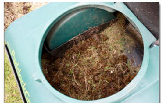
to the correct height for collection, then drive around your paddock over top of any horse poo and debris you wish to collect. When the tray is full, slide it out the back and empty the contents wherever you wish. Once finished cleaning your paddock, wind the handle back up to lift the brushes off the ground (so you are not continuing to sweep on your way back to parking area) and unhook your Paddock Groomer from the towing vehicle - it's that simple!
